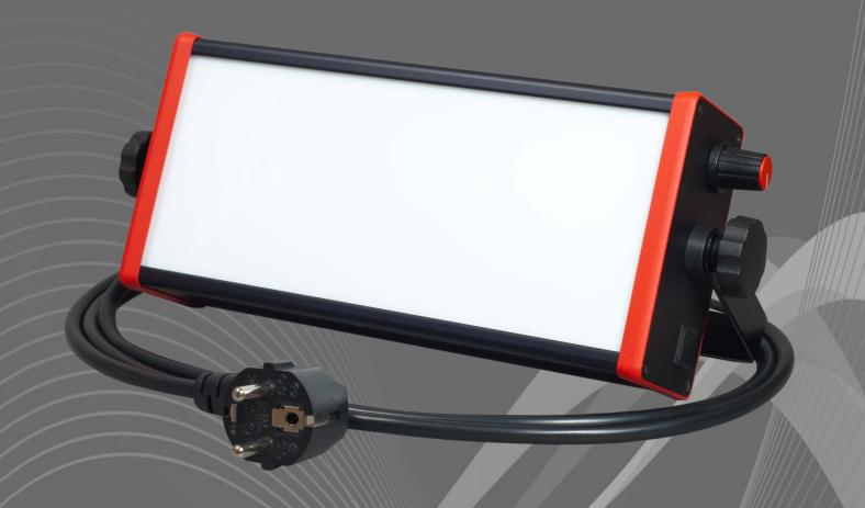
**Microprocessor animal-room lighting MLC-S V3 RAT** uses narrowband LEDs emission and is designed to illuminate the test site in the premises of the animal house, with recommended side wall mounting. The light source is 96 red SMD LEDs in triple PLCC6 enclosures, emitting a 660 nm light wave and a deep-red color.
